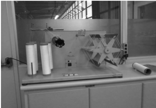
Figure 2 - ASPA - Apparatus for measuring the yarn count
